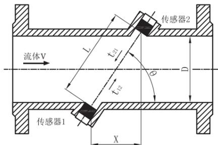
$$v = \frac{L}{2 \cos \theta} \left( \frac{1}{t_{12}} - \frac{1}{t_{21}} \right) \quad (\text{式1})$$
